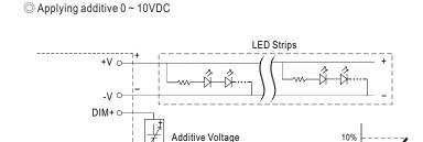
"DO NOT connect "DIM- to -V"
