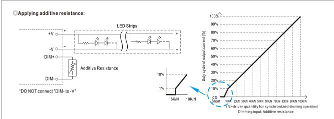
Note: 1. Min. duty cycle of output current is about 1%, and the dimming input is about  $6K\Omega$  or 0.6VDC, or 10V PWM signal with 6% duty cycle. 2. The duty cycle of output current could drop down to 0% when dimming input is less than  $6K\Omega$  or less than 0.6VDC, or 10V PWM signal with duty cycle less than 6%.
